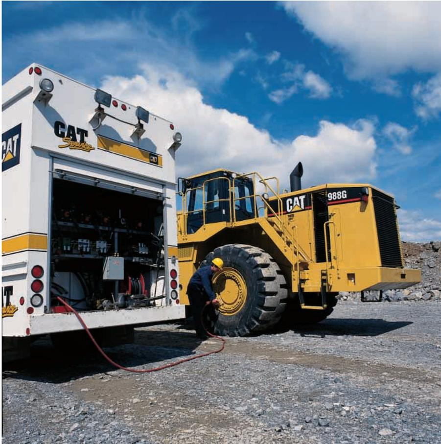
**Maintenance and Repair.** Is easier through monitoring key functions and logging critical indicators. Electronic diagnostic access is possible with a single tool, the Electronic Technician (ET). In addition to the servicing features built into the engine, the 988G includes:
