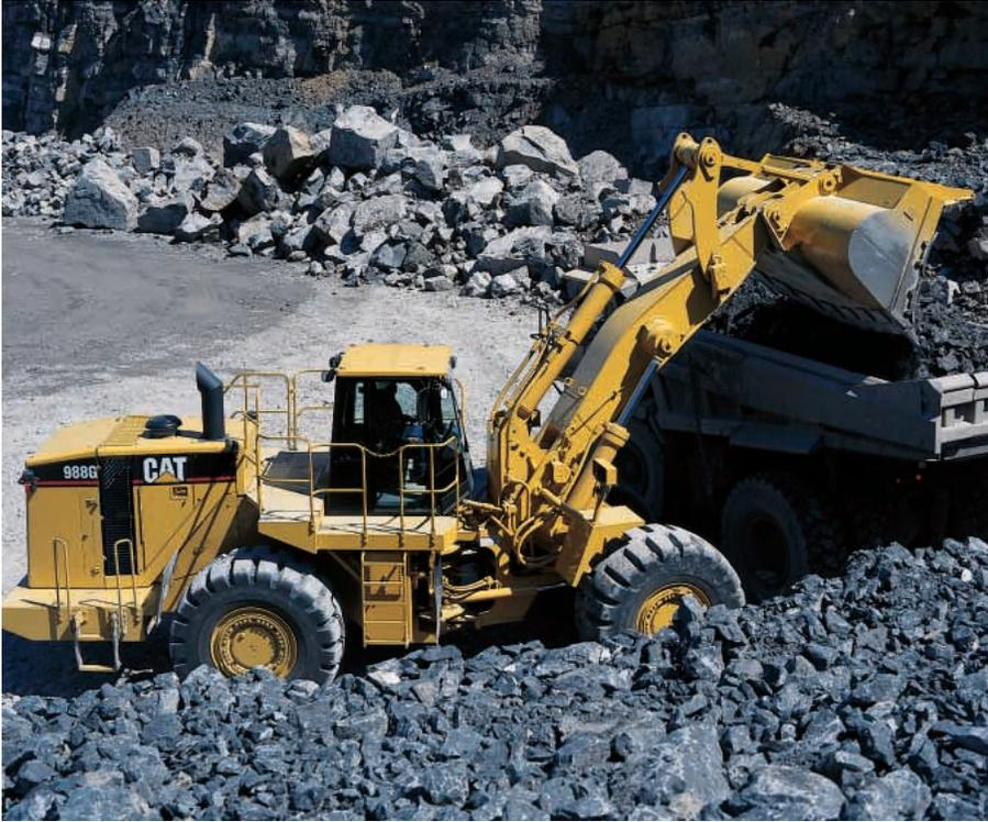
**Performance.** The 988G is an aggressive first gear loader for face and bank excavation. With increased dump clearance, the 988G can easily load 37-63 tonnes (40 to 70 ton) off-highway trucks. Increased performance and good pass match make the 988G a versatile performer with a cost per ton that will help your bottom line.
