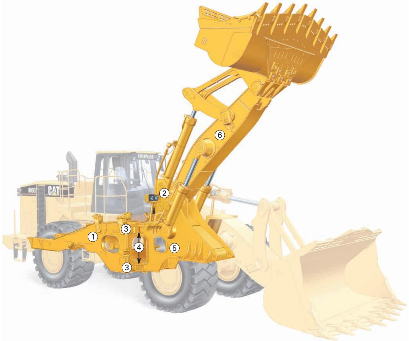
**Structures.** Combine the use of robotic welding and castings in critical high-stress areas. More than 90 percent of the 988G structure is robotically welded to provide highly consistent welds and increased strength. Castings are also used in several areas to increase strength by helping to spread the loads and reduce the number of parts.
