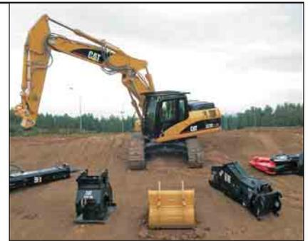
**Work Tools.** Choose from a variety of work tools such as hammers, crushers, pulverizers, shears, multi-processors and grapples.
