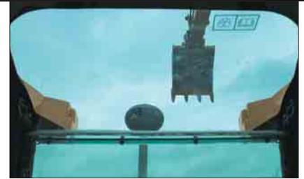
**Skylight.** A unique large polycarbonate skylight provides very good upward visibility, especially useful in above ground applications.
