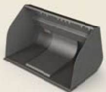
Light material bucket with bolt-on edges
