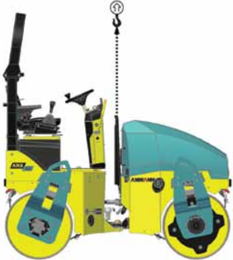
Central lifting point on ARX1(standard) ARX2(option)
