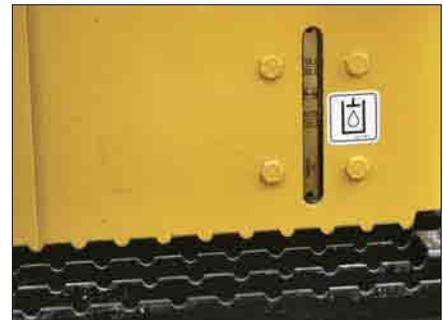
**Sight Gauges.** Well-protected, yet easily visible sight gauges for the transmission oil, hydraulic oil and engine coolant allow easy daily checks while reducing the risk of contaminants entering the systems.
