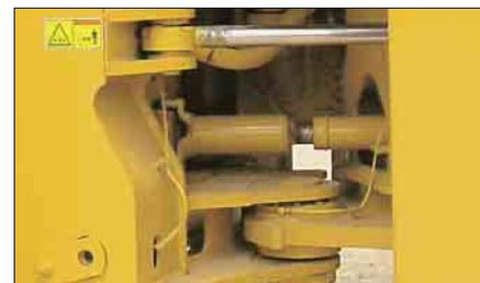
**Spread Hitch.** The distance between the upper and lower hitch plates is important for machine performance and component life. The Cat spread hitch design provides excellent load distribution and bearing life. Both the upper and lower hitch pins pivot on double tapered roller bearings – improving durability by distributing both vertical and horizontal loads over a larger surface area. The wide opening also provides excellent service access.
