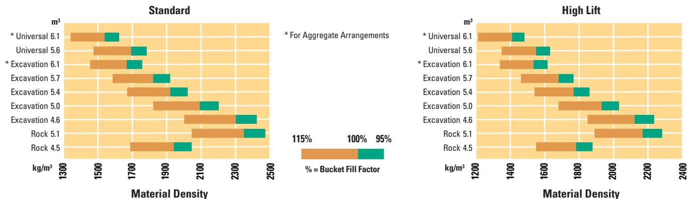
In accordance with SAE J818, these data consider the bucket load to be equal to half of the static tipping load at full turn.
