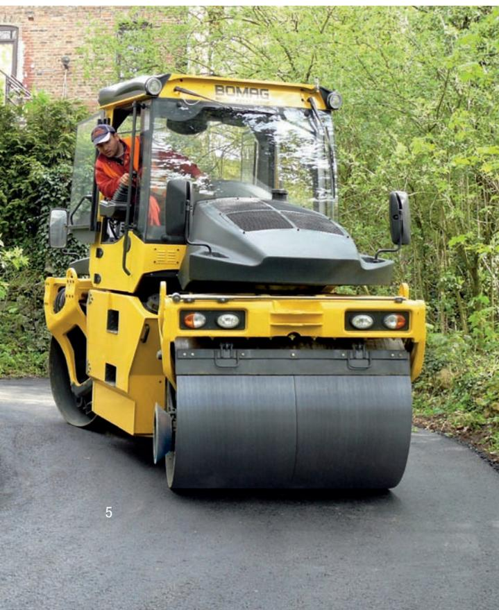
Split drums reduce shearing stresses around tight curves, and the potential for asphalt surface tearing is reduced.
