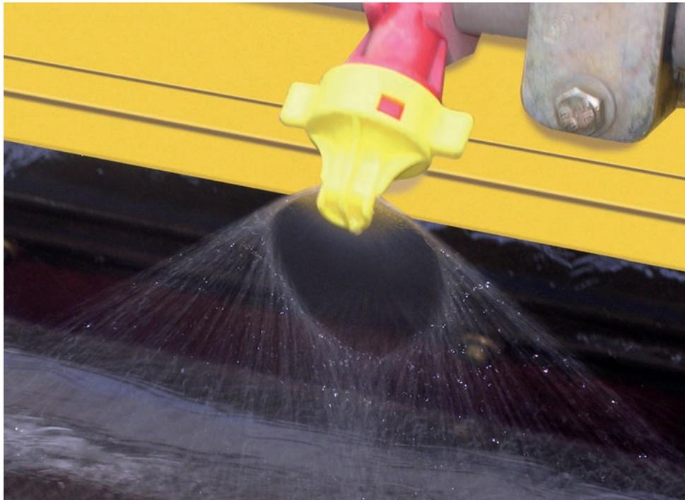
High-performance nozzles provide even spray to the drum surface.
