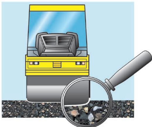
Special drum geometry produces seamless transition points
