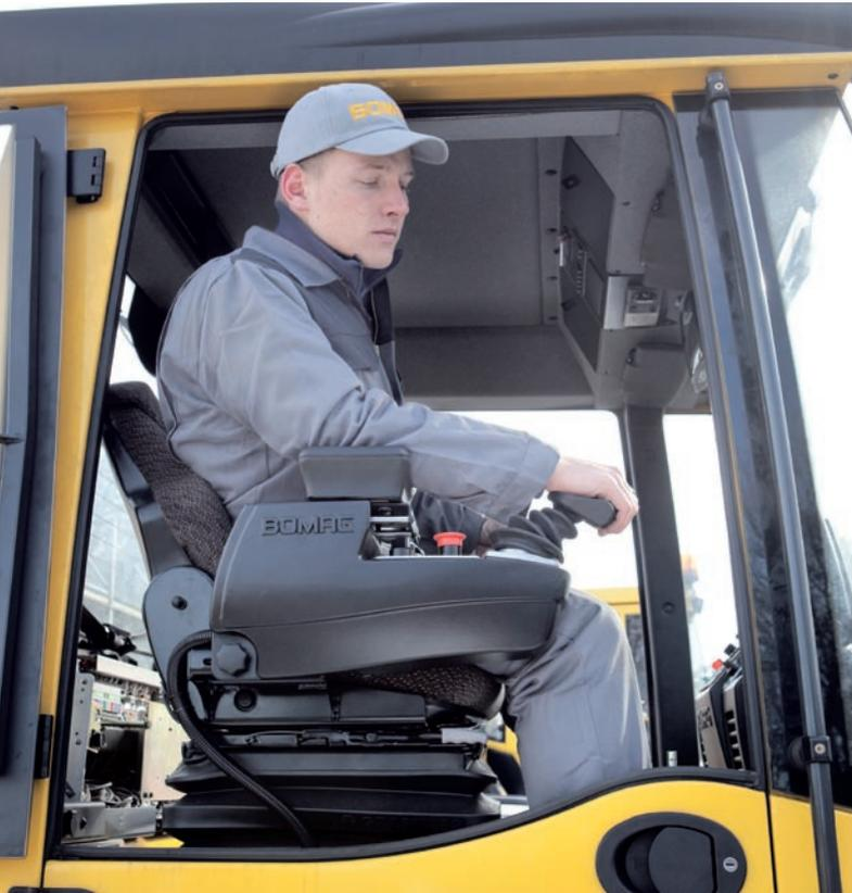
The foot-operated seat can be easily shifted across a wide range – the armrest projects out of the window at the extreme limit.
