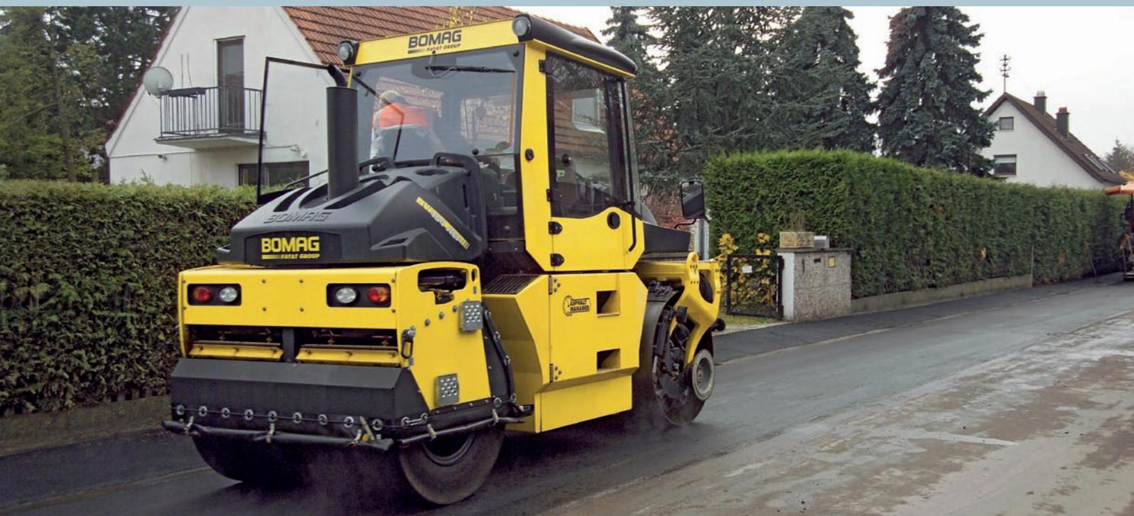
BOMAG also offers all pivot-steered asphalt rollers as an ACP combination version for careful rolling and kneading effect on asphalt.
