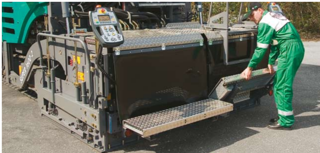
The split footboard of the screed folds up easily for transport.
