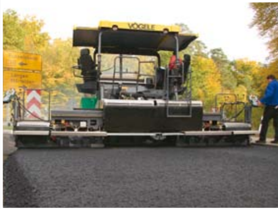
AB 500 TV built up to maximum pave width
