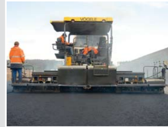
AB 600 TV built up to maximum pave width
