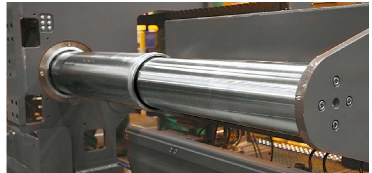
Amplly dimensioned, sturdy telescoping tubes featuring high-precision operation. They provide for excellent stability of the screed.
