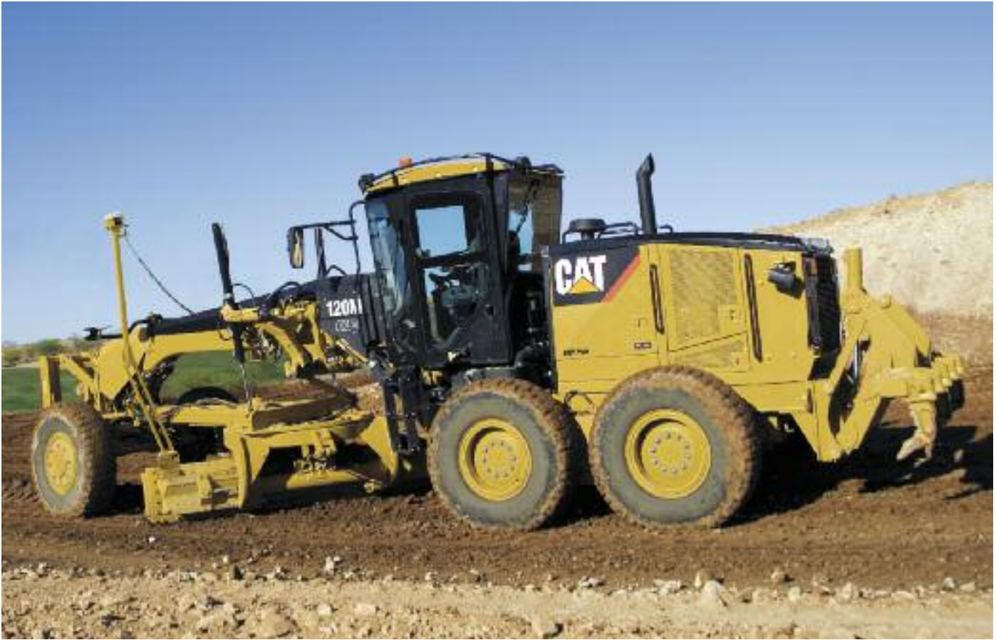
120M with AccuGrade™ System
